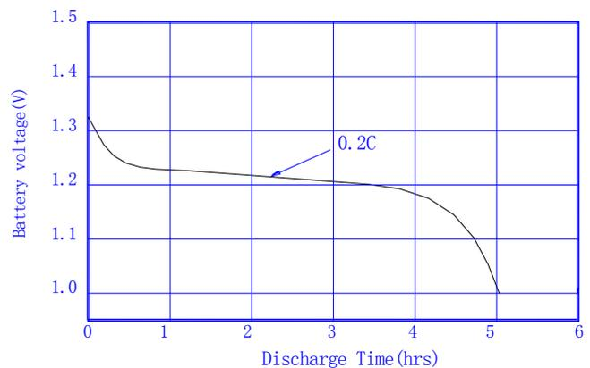
Typical Discharge curve (at 0.2C 20±5°C)
