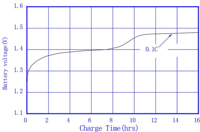
Typical charge curve (at 0.1C 20±5°C)
